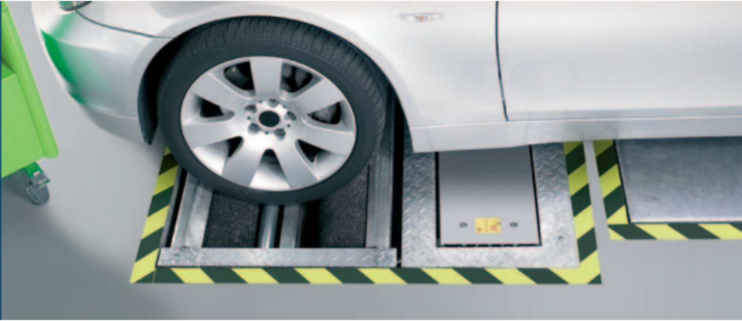
Complete: Modern passenger car brake testing system, test lane SDL 43xx
